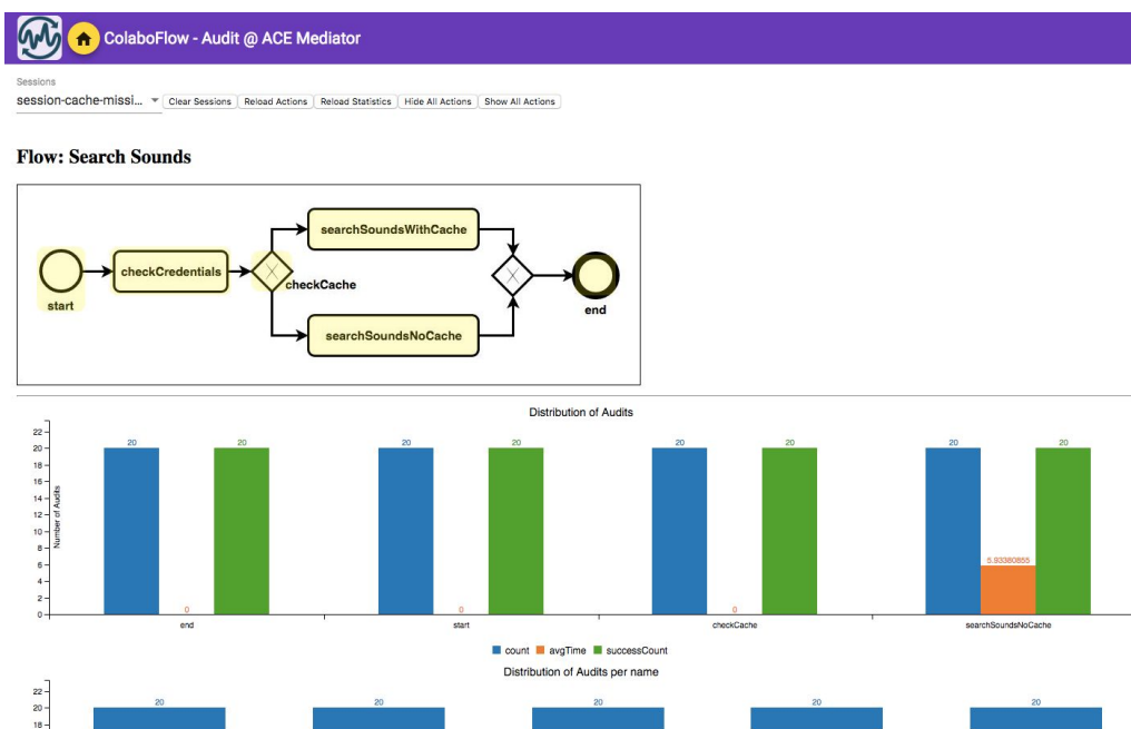
Figure 2.8.1. Example of the mediator's "Search Sounds" workflow analysis with its actions stats
