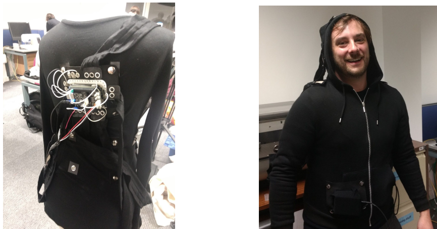
Figure 5. Sonic e-textile prototypes: Bela platform (left) and integration in hoodie (right)
