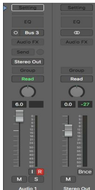
Figure 10 - Inserting auxiliary track via a bus to an audio track in Logic Pro X.
