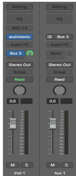
Figure 9 - Routing audio output to an auxiliary bus in Logic Pro X.
